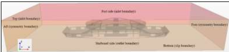
Figure 4. CFD analysis control volume for Üçkuyular-Bostanlı voyage.
