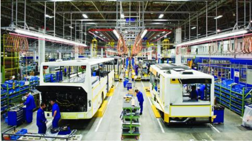
Figure 1: The bus assembly line (Mercedes Benz-Istanbul, https://busride.com/wp-content/uploads/2012/05/web-LFE-turkey1.jpg )
